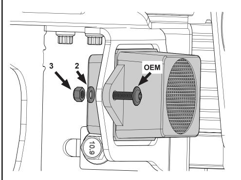
NOTE: ALIGN TABS ON SPEAKER WITH SMALLER HOLES IN SPEAKER BRACKET
